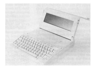
The Commodore LCD Personal Computer can run on 4 AA alkaline batteries for 15 hours.
